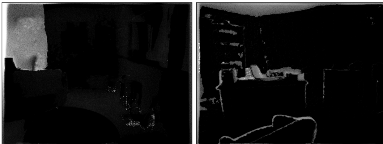
Figure B-1. Error Masks. The absolute distance errors for two scenes from the NYUv2 dataset show depth errors around object edges. Brighter pixels show higher absolute error for memory foveation.
